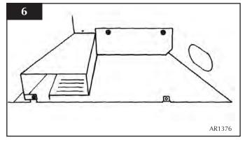
1.18 Inspect the space behind the fireplace for debris and the condition of the chimney, the flue flow test should be carried out now. Remove any debris and carry out any necessary remedial work.
